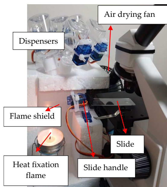
Figure 4. Parts of the automated sample processor prototype. The servomotors' arms of the dispensers are attached to a rubber piece to open and close the pressure relief hole on the top of each container, as required for solution flow from the hole in the bottom. Five dispensers are used for crystal violet, iodine, ethyl alcohol, safranin, and distilled water for washing between staining stages.
